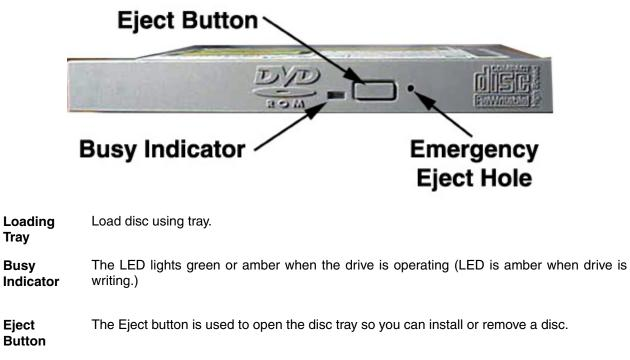
**Emergency** The emergency eject hole is to be used only when the Loading Tray will not open when Eject button is pressed.
